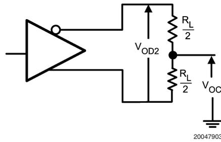
FIGURE 1. Test Circuit for  $V_{OD2}$  and  $V_{OC}$
