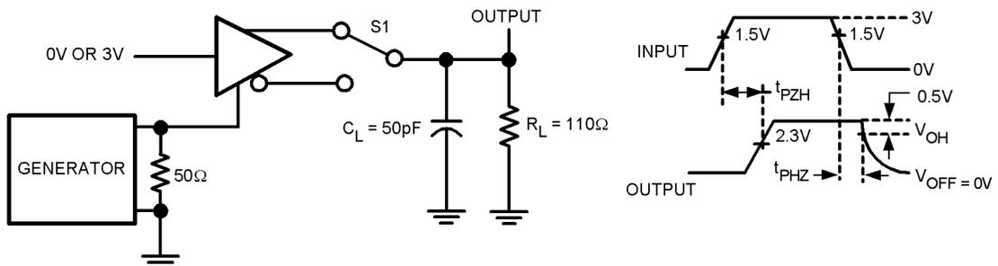
FIGURE 4. Test Circuit for Driver  $T_{PZH}$  and  $T_{PHZ}$
