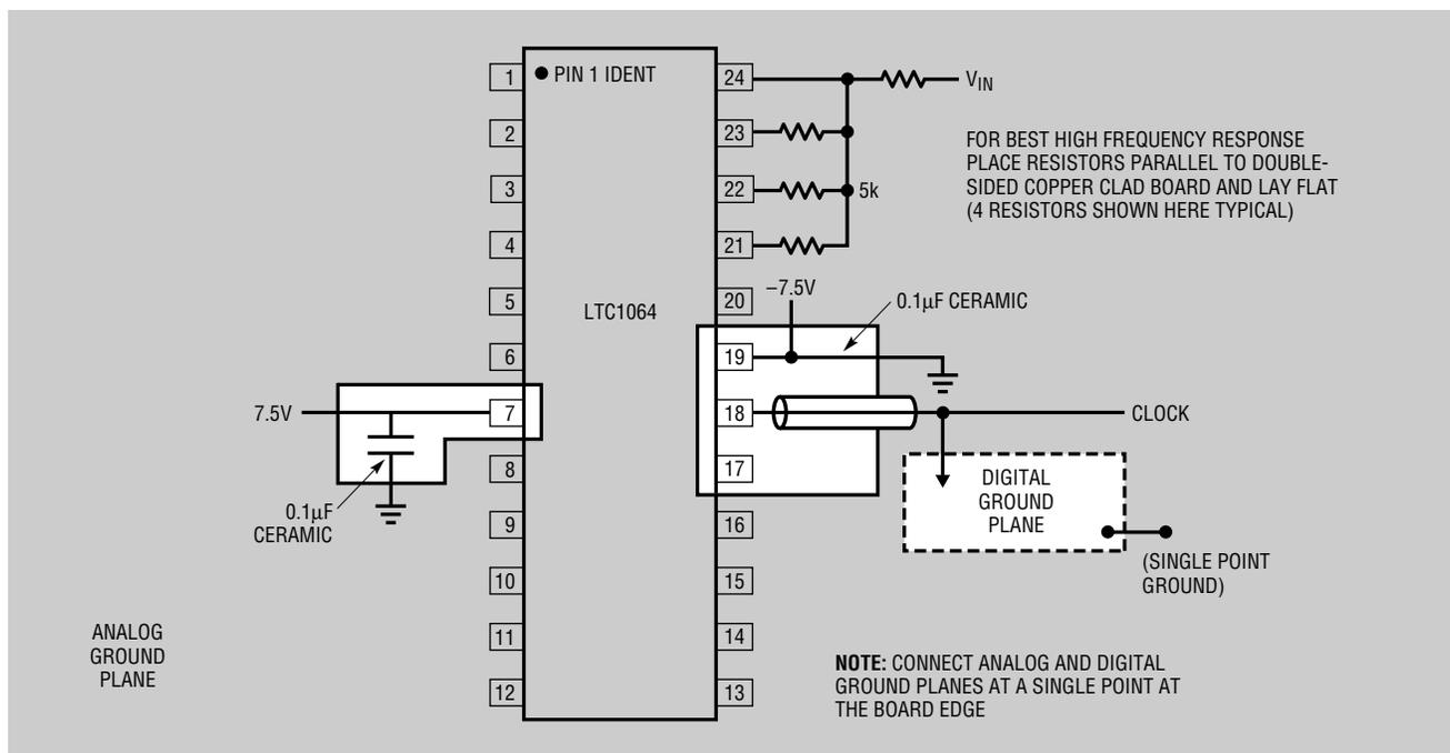
Figure 2. Example Ground Plane Breadboard Technique for LTC1064
