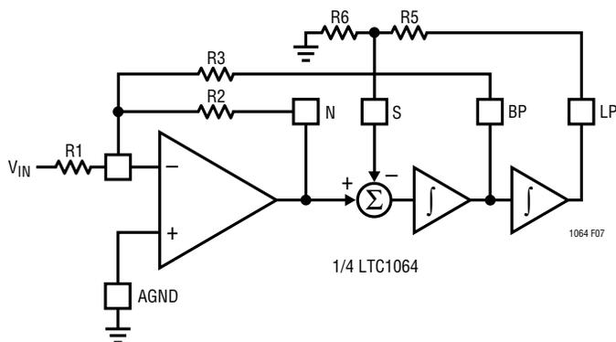
$$\begin{aligned} f_0 &= \frac{f_{\text{CLK}}}{100(50)} \sqrt{\frac{R_6}{R_5 + R_6}}; f_n = f_0; Q = \frac{R_3}{R_2} \sqrt{\frac{R_6}{R_5 + R_6}}; \\ H_{\text{ON1}}(f \rightarrow 0) &= H_{\text{ON2}} \left( f \rightarrow \frac{f_{\text{CLK}}}{2} \right) = -\frac{R_2}{R_1}; H_{\text{OLP}} = -\frac{R_2}{R_5 + R_6}; \\ H_{\text{OBP}} &= -\frac{R_3}{R_1}; R_5 || R_6 \leq 5k \end{aligned} \quad 1064 \text{ F07 Eq}$$
