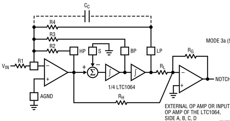
$$\text{MODE 3a (100:1): } f_0 = \frac{f_{\text{CLK}}}{100} \sqrt{\frac{R_2}{R_4}}; f_n = \frac{f_{\text{CLK}}}{100} \sqrt{\frac{R_H}{R_L}}; H_{\text{OHP}} = -\frac{R_2}{R_1}; H_{\text{OBP}} = -\frac{R_3}{R_1};$$
