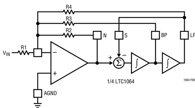
$$\text{MODE 2 (100:1): } f_0 = \frac{f_{\text{CLK}}}{100} \sqrt{1 + \frac{R_2}{R_4}}; f_n = \frac{f_{\text{CLK}}}{50}; Q = \frac{R_3}{R_2} \sqrt{1 + \frac{R_2}{R_4}}; H_{\text{OLP}} = -\frac{\frac{R_2}{R_1}}{1 + \frac{R_2}{R_4}}$$
