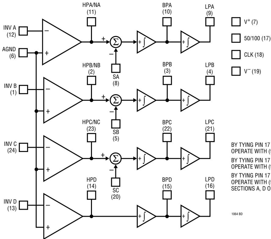
BY TYING PIN 17 TO V<sup>+</sup>, ALL SECTIONS OPERATE WITH (f<sub>CLK</sub>/f<sub>0</sub>) = 50:1.
