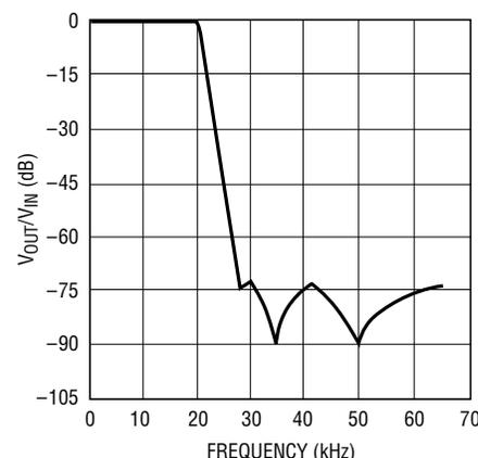
8TH ORDER CLOCK-SWEEPABLE LOWPASS ELLIPTIC ANTIALIASING FILTER MAINTAINS, FOR  $0.1\text{Hz} \leq f_{CUTOFF} \leq 20\text{kHz}$ , A  $\pm 0.1\text{dB}$  MAX PASSBAND ERROR AND 72dB MIN STOPBAND ATTENUATION AT  $1.5 \times f_{CUTOFF}$ .
