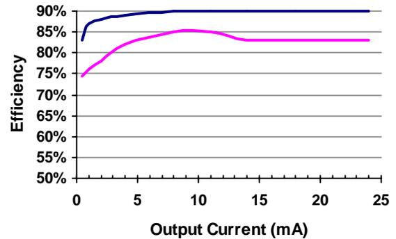
**Figure 13** – LED Driver (Upper) and LCD Bias Efficiency
