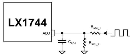
**Figure 5 – LCD Bias Adjustment Input Filter**
