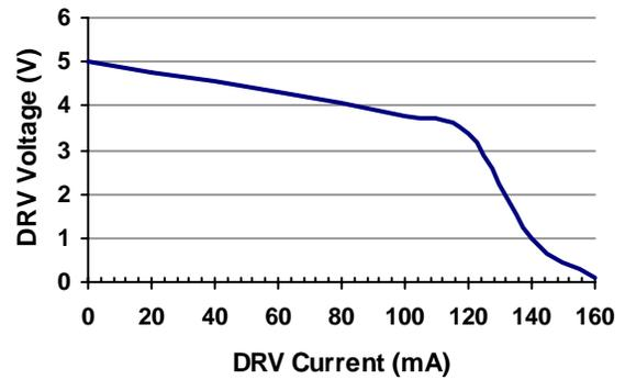
**Figure 11** – Gate Drive Voltage Vs. Drive Current
