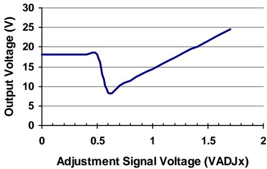
**Figure 10** – Output Voltage Vs. Adjustment Signal Threshold
