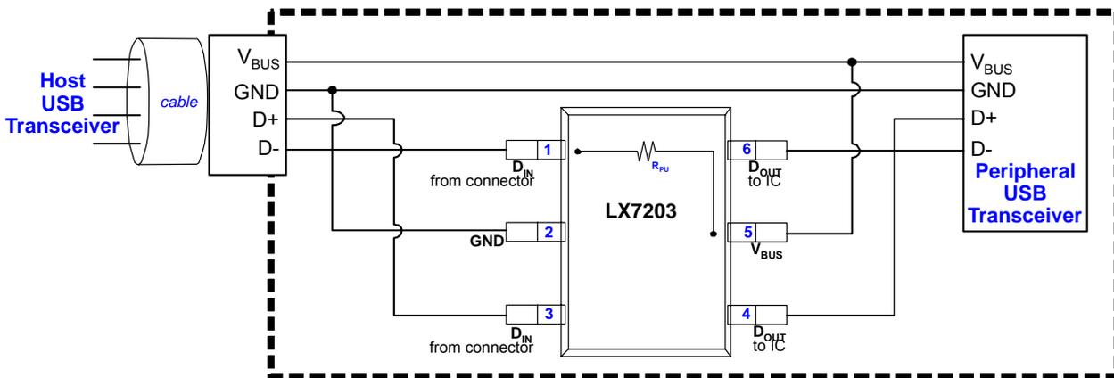
**Figure 3 – Connection for Low Speed Operation**
