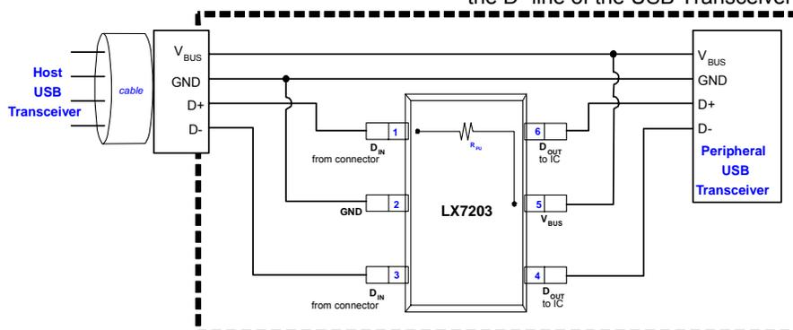
**Figure 2 – Connection for Full Speed Operation**
