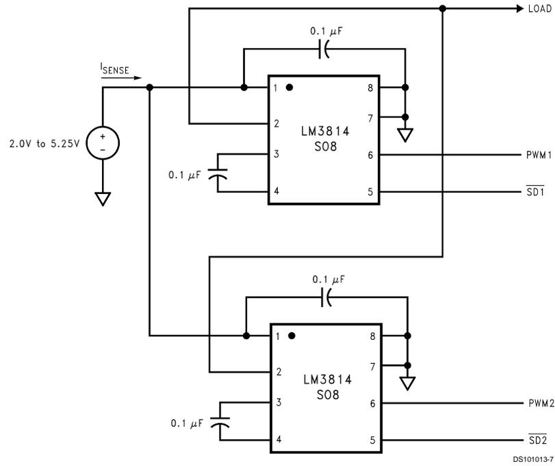
**FIGURE 3. Paralleling LM3814 for Higher Load Current**
