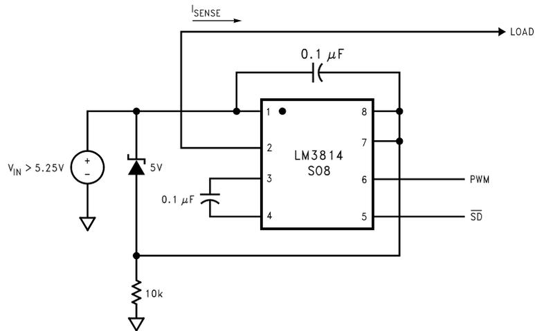
**FIGURE 4. High Voltage Operation —  $V_{IN}$  Greater Than 5.25V (High Side Sense)**
