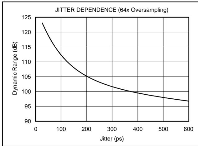
FIGURE 16. Jitter Sensitivity.
