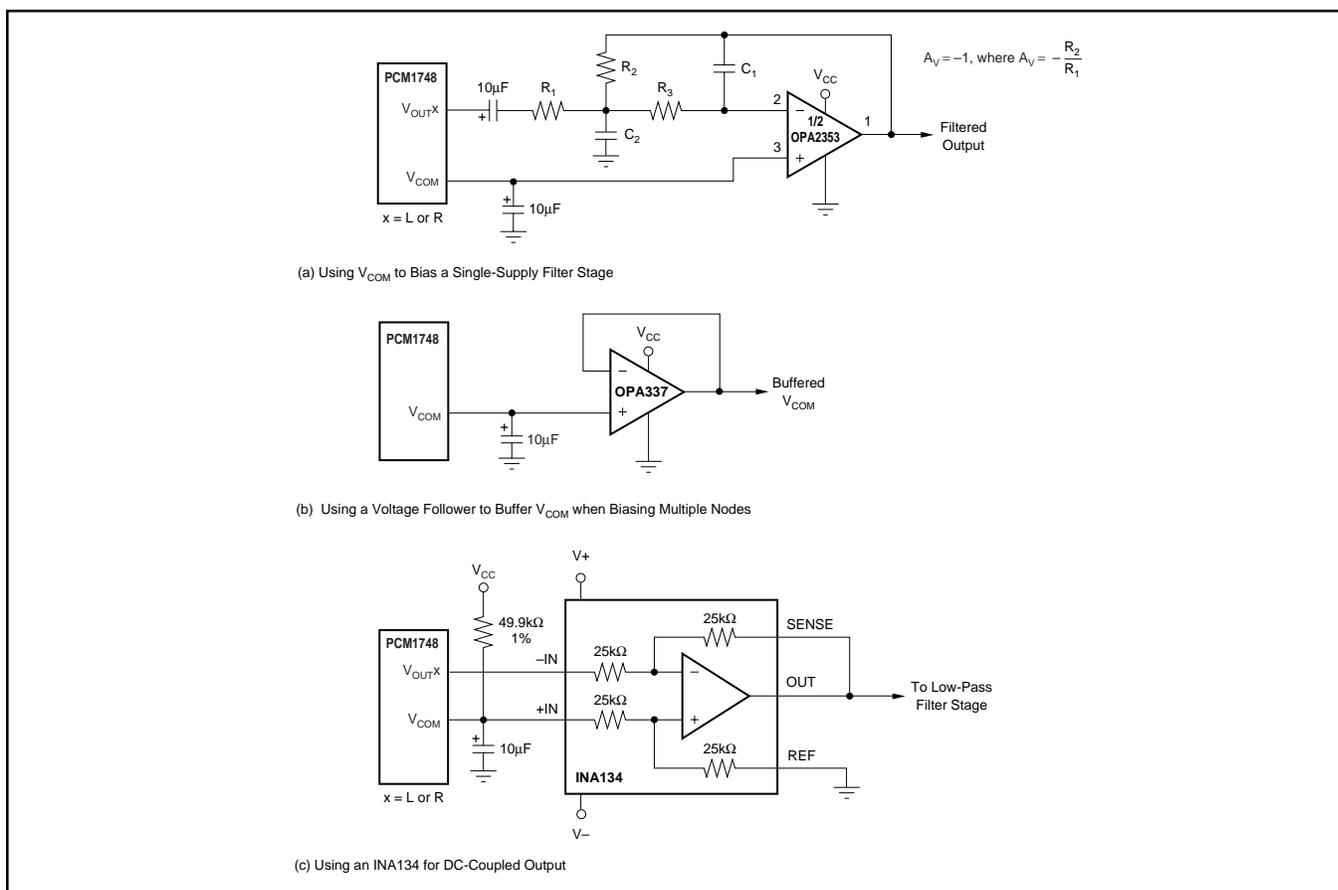
FIGURE 9. Biasing External Circuits Using the  $V_{COM}$  Pin.
