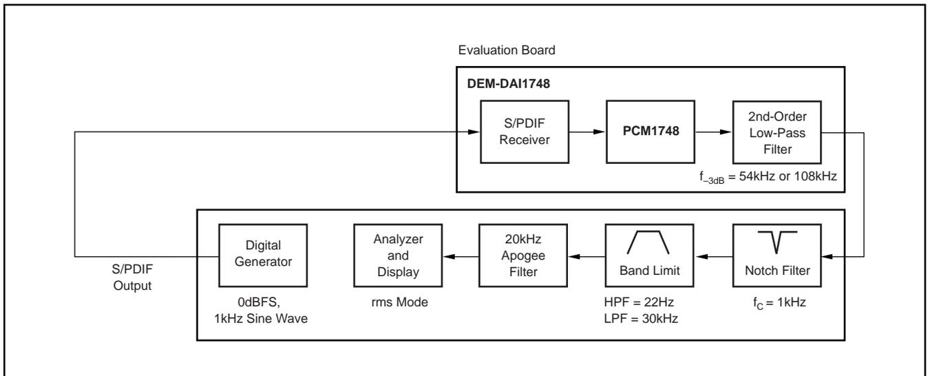
FIGURE 17. Test Setup for THD+N Measurements.
