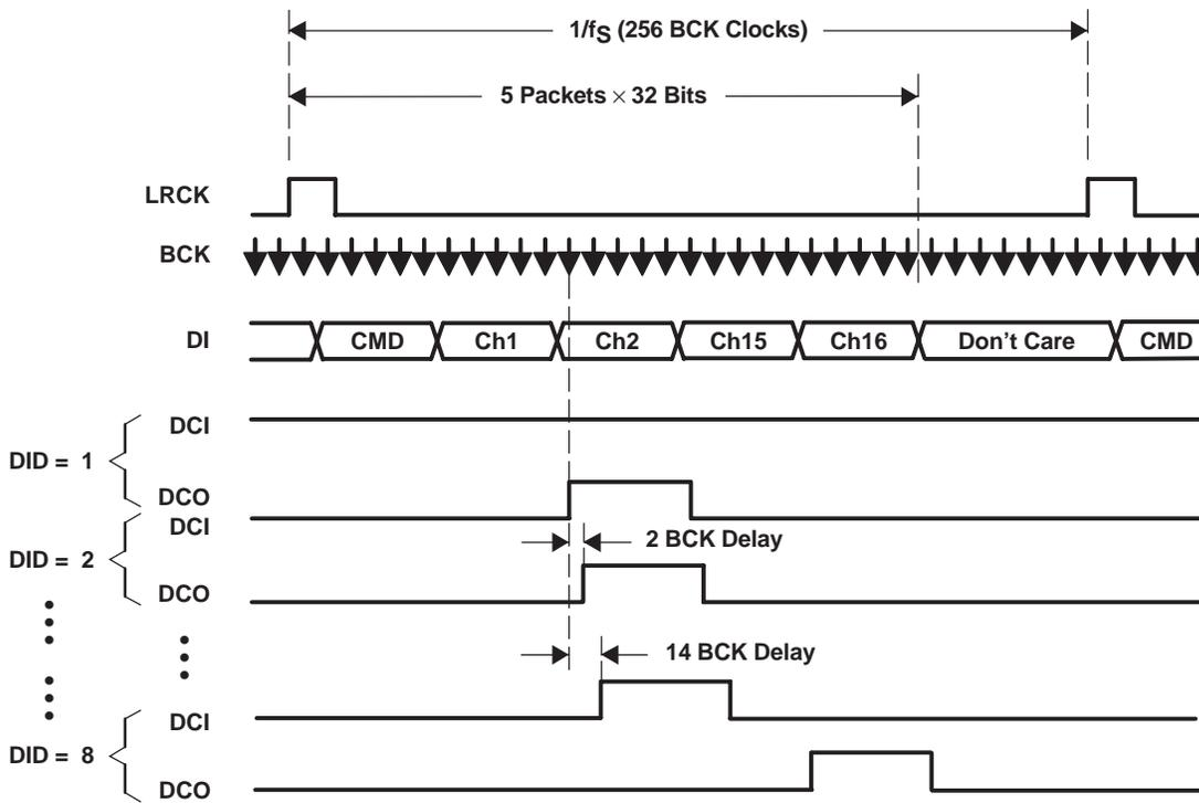
Figure 61. DCO Output Timing With Skip Operation
