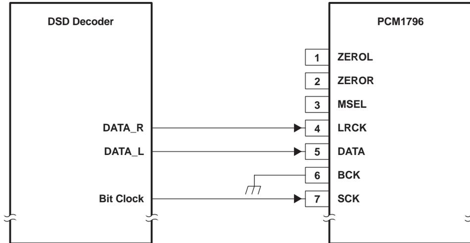
**Figure 42. Connection Diagram in DSD Mode**
