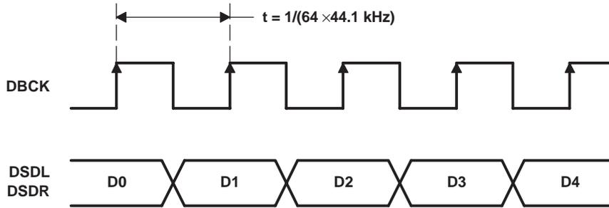
**Figure 43. Normal Data Output Form From DSD Decoder**
