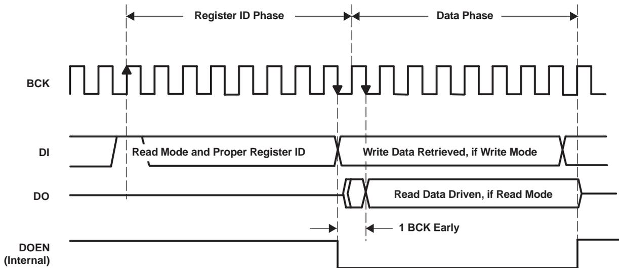
**Figure 59. TDMCA Write and Read Operation Timing**
