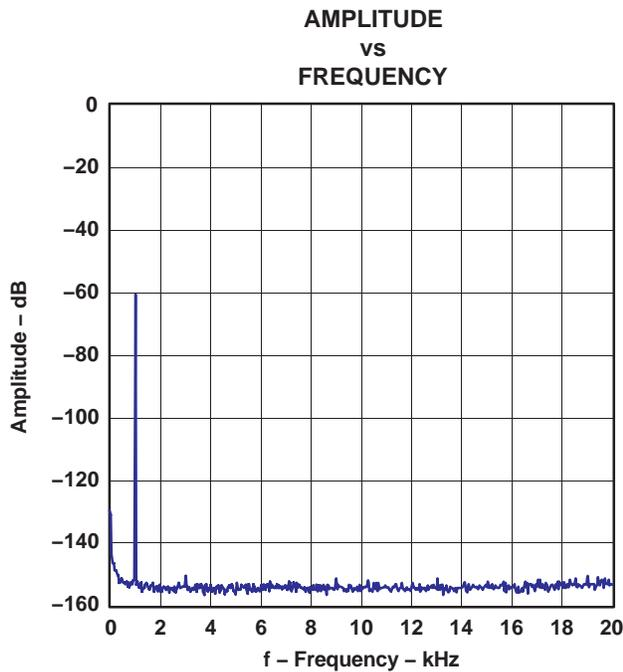
NOTE: PCM mode,  $f_S = 48$  kHz, 32768 point 8 average,  $T_A = 25^\circ\text{C}$ ,  $V_{DD} = 3.3$  V  $V_{CC} = 5$  V, measurement circuit is Figure 36.
