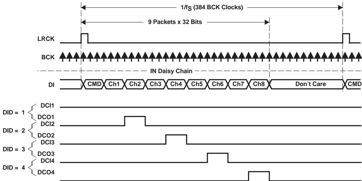
Figure 60. DCO Output Timing of TDMCA Mode Operation
