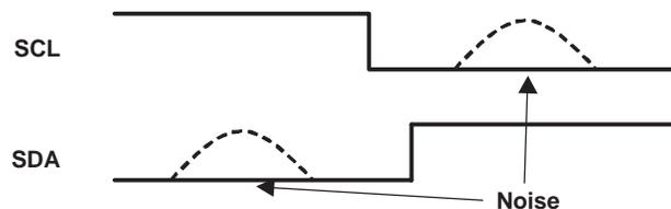
When these conditions occur at the same time, the PCM1796 erroneously detects a start or stop condition.
