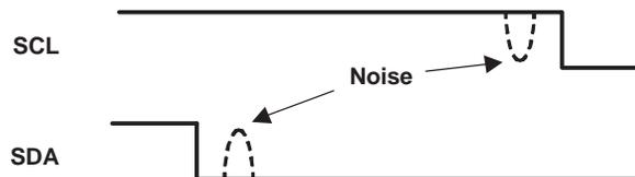
When these conditions occur at the same time, the PCM1796 fails to detect a start condition.
