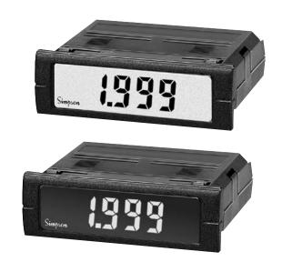
Simpson's Mini-Max Voltage Indicators provide high quality, accuracy, and reliability in a compact, 60mm deep case. Units offer 3-1/2 digit, 0.5" (12.7mm) LCD display and are available with a bright red, negative image backlight option. All units feature user-selectable decimal point, auto zero and limited scaling capabilities.
