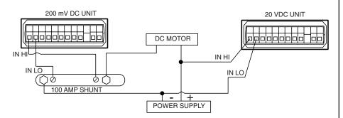
lead of the shunt is connected to the IN HI terminal, and the negative lead connected to the IN LO terminal.
