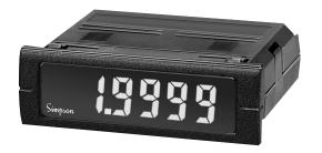
Simpson's Mini-Max Voltage Indicators provide high quality, accuracy and reliability in a compact, 60mm deep case. Units offer 4-1/2 digit, 0.5" (12.7mm) LCD display and are available with a bright red, negative image backlight option. All units feature user-selectable decimal point, auto zero and limited scaling capabilities.
