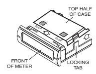
Using a screwdriver or thumbnail, spread tab on each side of case to unlock top half. Lift rear top half and slide away from front of meter.
