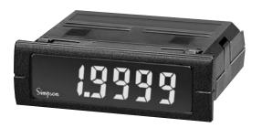
Simpson's Mini-Max Voltage Indicators provide high quality, accuracy and reliability in a compact, 60mm deep case. Units offer 4-1/2 digit, 0.5" (12.7mm) LCD display and are available with a bright red, negative image backlight option. All units feature user-selectable decimal point, auto zero and limited scaling capabilities.
