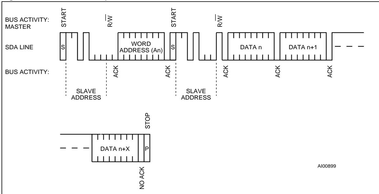
Figure 13. Alternate READ Mode Sequence
