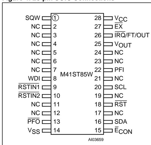
Figure 5. 28-pin, 300mil SOIC (MX) Connections
