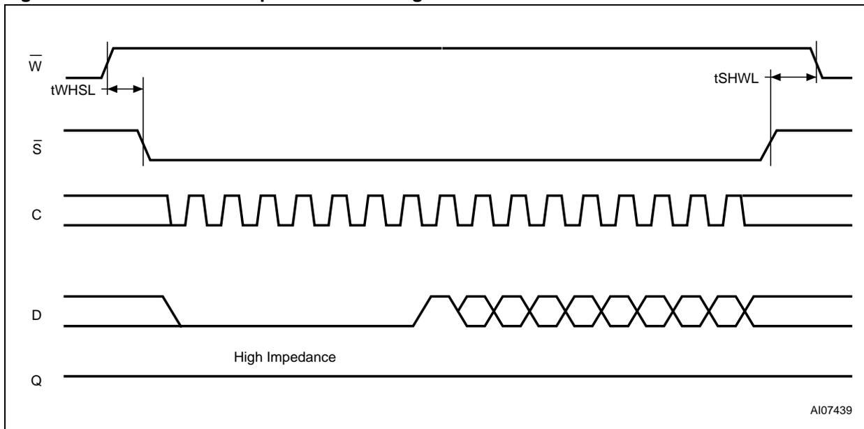
Figure 24. Output Timing
