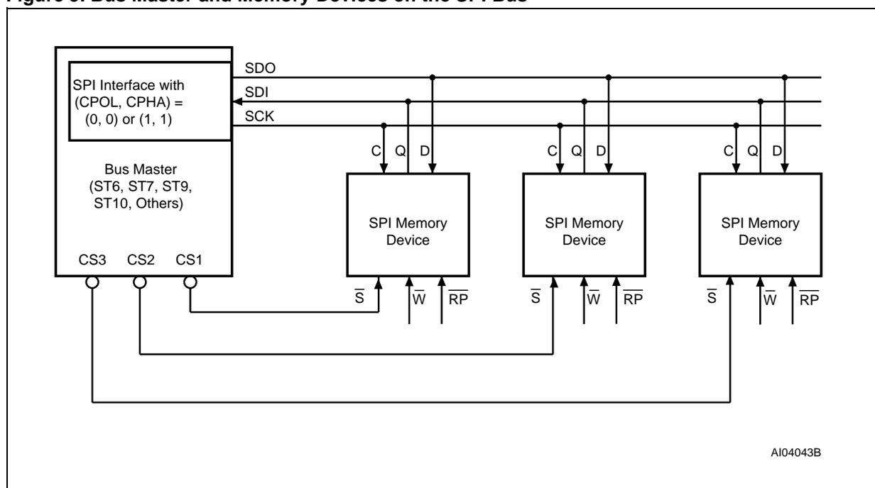
Note: The Write Protect ( $\bar{W}$ ) signal should be driven, High or Low as appropriate.
