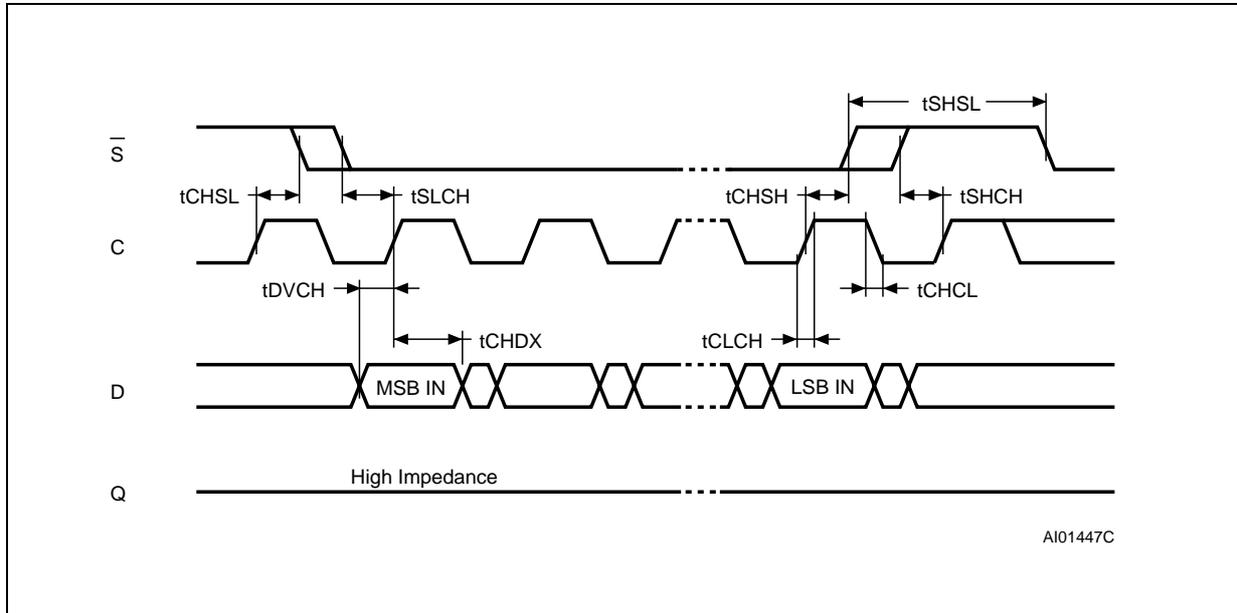
Figure 23. Write Protect Setup and Hold Timing
