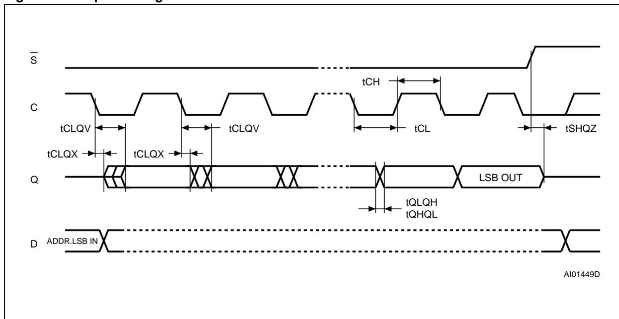
Figure 25. Reset AC Waveforms
