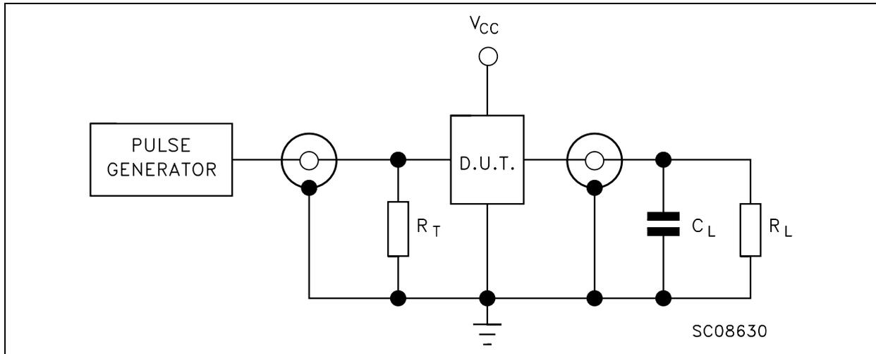
$C_L = 50\text{pF}$  or equivalent (includes jig and probe capacitance)
