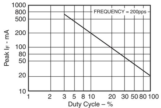
Fig. 3D. Max Peak Current vs. Duty Cycle
