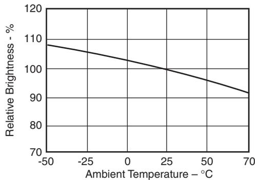
Fig. 1C. Relative Luminous Intensity vs. Temperature
