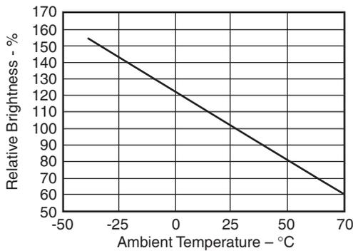
Fig. 3C. Relative Luminous Intensity vs. Temperature (See Note 2)
