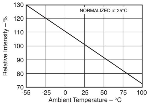
Fig. 2C. Relative Luminous Intensity vs. Temperature (See Note 2)
