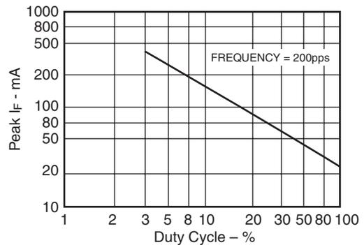
Fig. 1D. Max Peak Current vs. Duty Cycle
