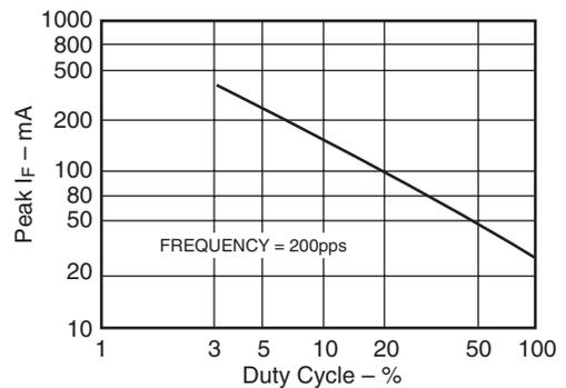
Fig. 4D. Maximum Peak Current vs. Duty Cycle
