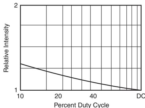
Fig. 3E. Relative Luminous Intensity vs. Duty Cycle
