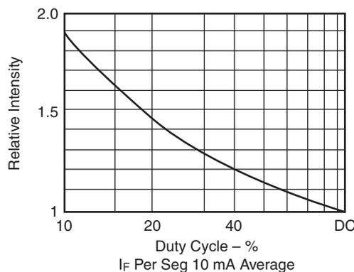
Fig. 1E. Relative Luminous Intensity vs. Duty Cycle
