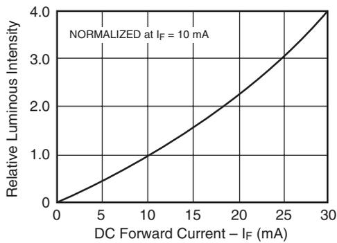
Fig. 4A. Relative Luminous Intensity vs. Forward Current
