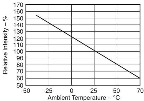
Fig. 3C. Relative Luminous Intensity vs. Temperature
