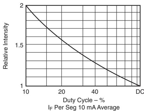
Fig. 4E. Relative Luminous Intensity vs. Duty Cycle
