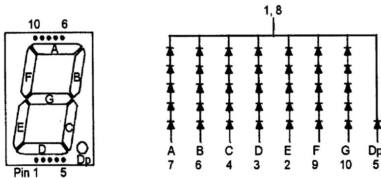
**GRAPHICAL DETAIL: AlGaAs Red** ( $T_A = 25^\circ\text{C}$  unless otherwise specified)
