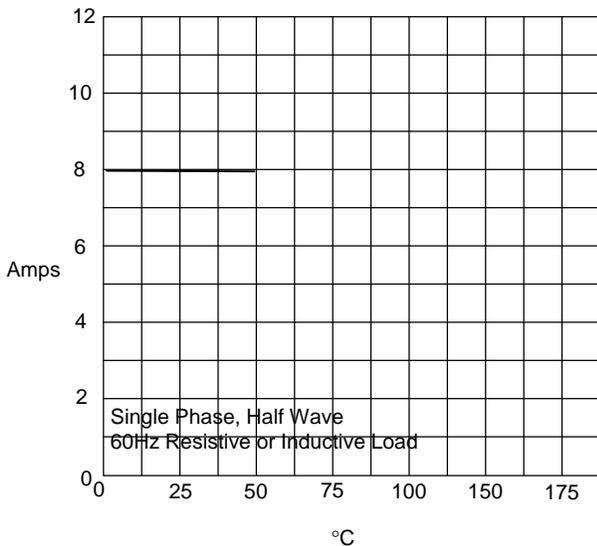
Average Forward Rectified Current - Amperes versus
