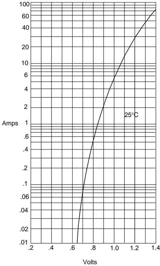
Instantaneous Forward Current - Amperes versus
