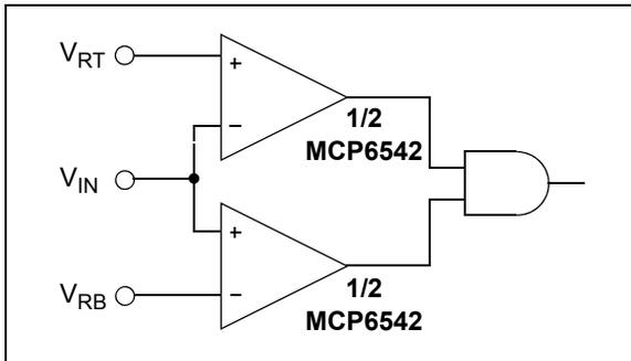
**FIGURE 4-10:** *Windowed Comparator.*
