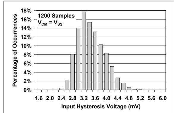
**FIGURE 2-4:** Input Hysteresis Voltage at  $V_{CM} = V_{SS}$ .
