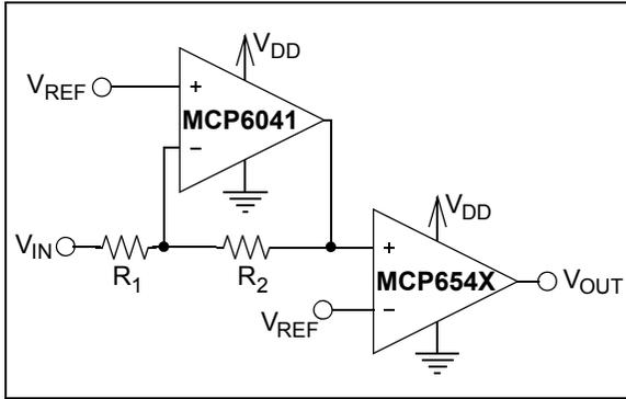
**FIGURE 4-9:** *Precise Inverting Comparator.*
