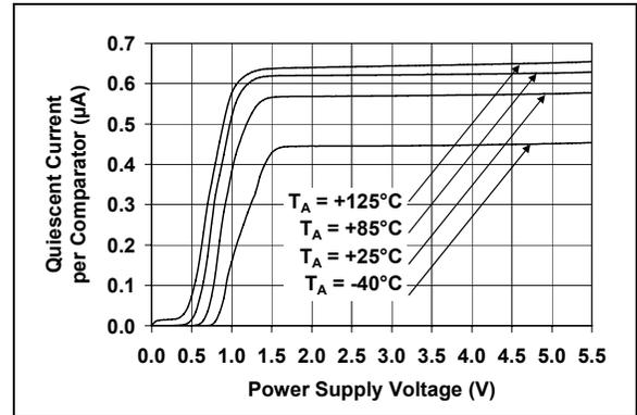
**FIGURE 2-17:** Quiescent Current vs. Power Supply Voltage.
