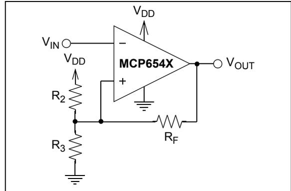
**FIGURE 4-5:** Inverting Circuit With Hysteresis.
