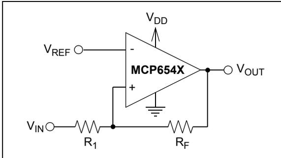
**FIGURE 4-3:** Non-inverting circuit with hysteresis for single-supply.
