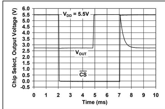
**FIGURE 2-34:** Chip Select ( $\overline{CS}$ ) Step Response (MCP6543 only).
