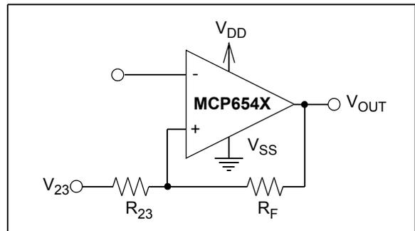
**FIGURE 4-7:** Thevenin Equivalent Circuit.
