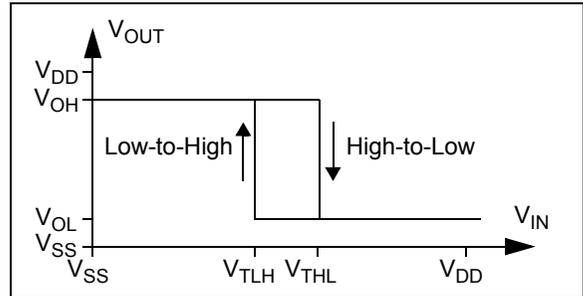
**FIGURE 4-6:** Hysteresis Diagram for the Inverting Circuit.
