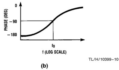
$$H_{HP}(s) = \frac{H_{OHP} s^2}{s^2 + \frac{s\omega_0}{Q} + \omega_0^2}$$
