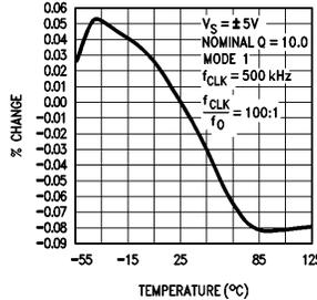
**f<sub>CLK</sub>/f<sub>0</sub> Deviation vs Temperature**
