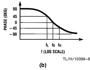
$$H_{BP}(s) = \frac{H_{OBP} \frac{\omega_0}{Q} s}{s^2 + \frac{s\omega_0}{Q} + \omega_0^2}$$
