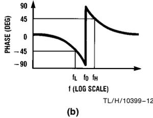
$$H_N(s) = \frac{H_{0N}(s^2 + \omega_0^2)}{s^2 + \frac{s\omega_0}{Q} + \omega_0^2}$$
