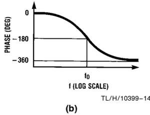
$$H_{AP}(s) = \frac{H_{0AP} \left( s^2 - \frac{s\omega_0}{Q} + \omega_0^2 \right)}{s^2 + \frac{s\omega_0}{Q} + \omega_0^2}$$
