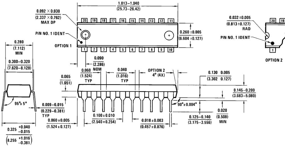
**20-Lead Molded Dual-In-Line Package (N)**
