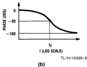
$$H_{LP}(s) = \frac{H_{OLP} \omega_0^2}{s^2 + \frac{s\omega_0}{Q} + \omega_0^2}$$
