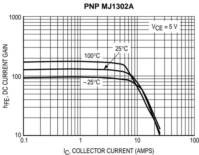
**Figure 5. DC Current Gain,  $V_{CE} = 5 V$**
