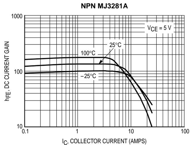
**Figure 6. DC Current Gain,  $V_{CE} = 5 V$**
