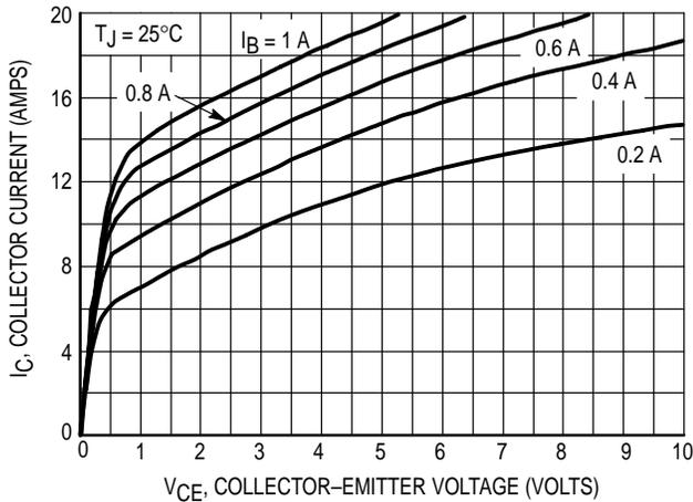
**Figure 9. Typical Output Characteristics**
