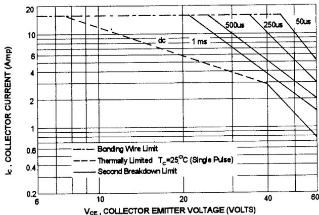
There are two limitation on the power handling ability of a transistor: average junction temperature and second breakdown safe operating area curves indicate  $I_C$ - $V_{CE}$  limits of the transistor that must be observed for reliable operation i.e., the transistor must not be subjected to greater dissipation than curves indicate.
