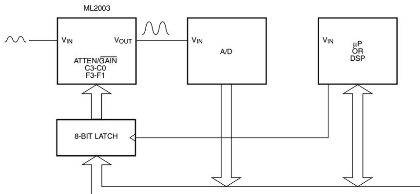
Figure 15. AGC for DSP or Modem Front End
