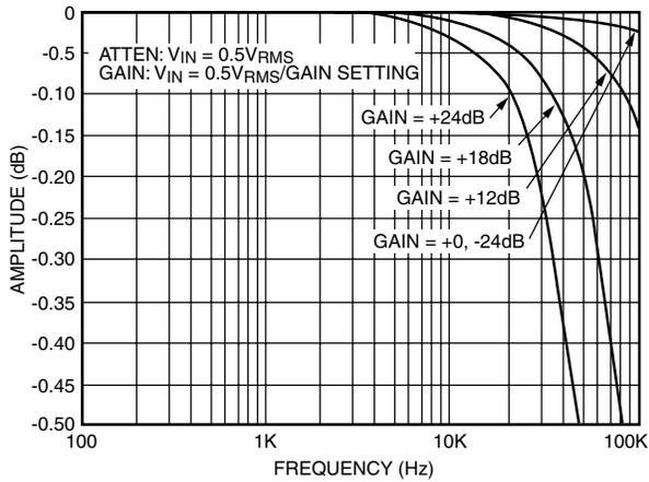
Figure 2. Amplitude vs Frequency ( $V_{IN}/V_{OUT} = .5V_{RMS}$ )
