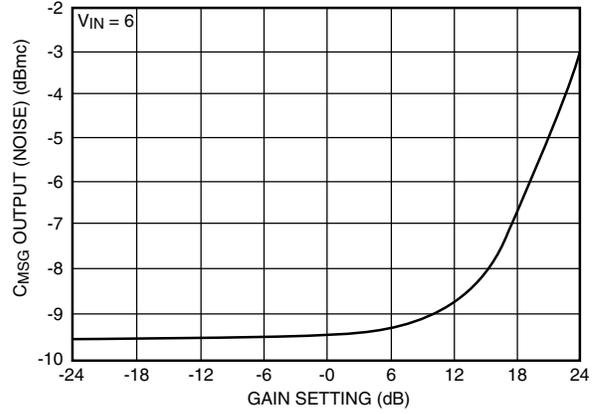
Figure 5. CMSG Output Noise vs Gain Settings
