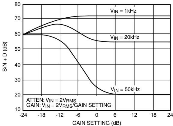
Figure 8. S/N + D vs Gain Setting (VIN/VOUT = 2VRMS)
