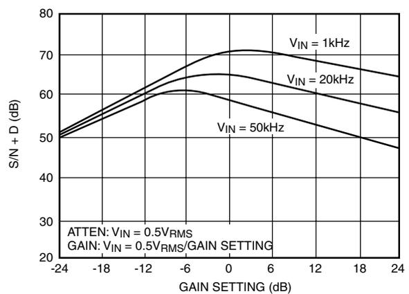
Figure 9. S/N + D vs Gain Setting (VIN/VOUT = 0.5VRMS)
