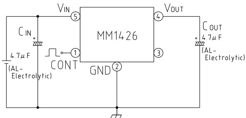
NOTE 1 : This regulator is not internally compensated and thus requires an external output-capacitor (C<sub>OUT</sub>) for stability.
