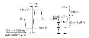
\*) total shunt capacitance of test jig and connectors
