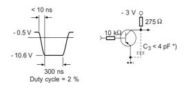
\*) total shunt capacitance of test jig and connectors
