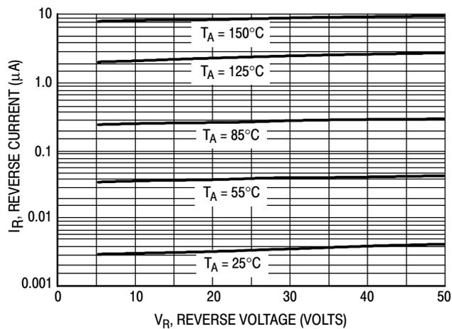
Figure 3. Leakage Current
