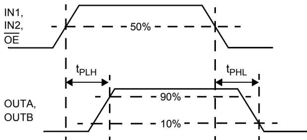
Figure 2.  $t_{PLH}$ ,  $t_{PHL}$ , and  $t_{PZH}$  Timing
