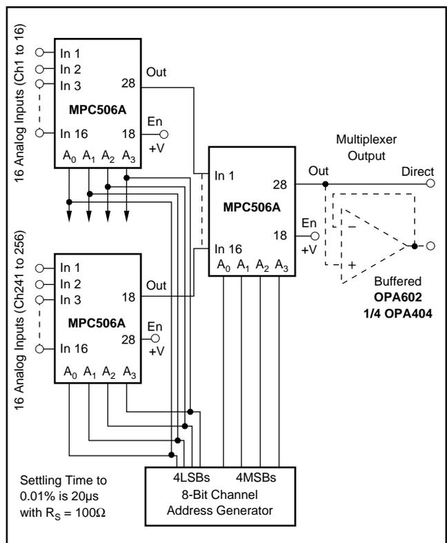
FIGURE 6. Channel Expansion up to 256 Channels Using  $16 \times 16$  Two-Tiered Expansion
