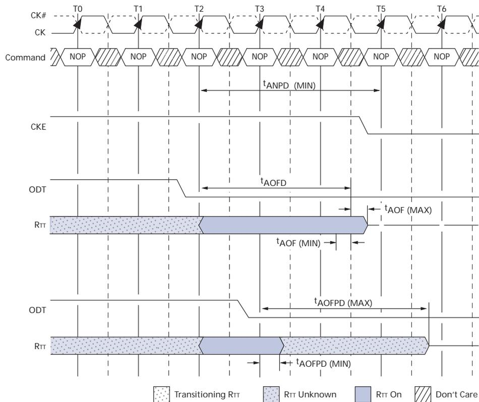
Figure 88: ODT Turn-On Timing When Entering Power-Down Mode
