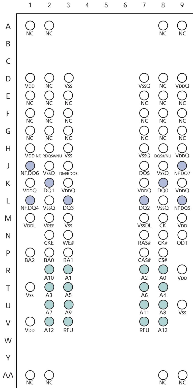
Figure 9: 92-Ball FBGA – x16 Ball Assignments (Top View)
