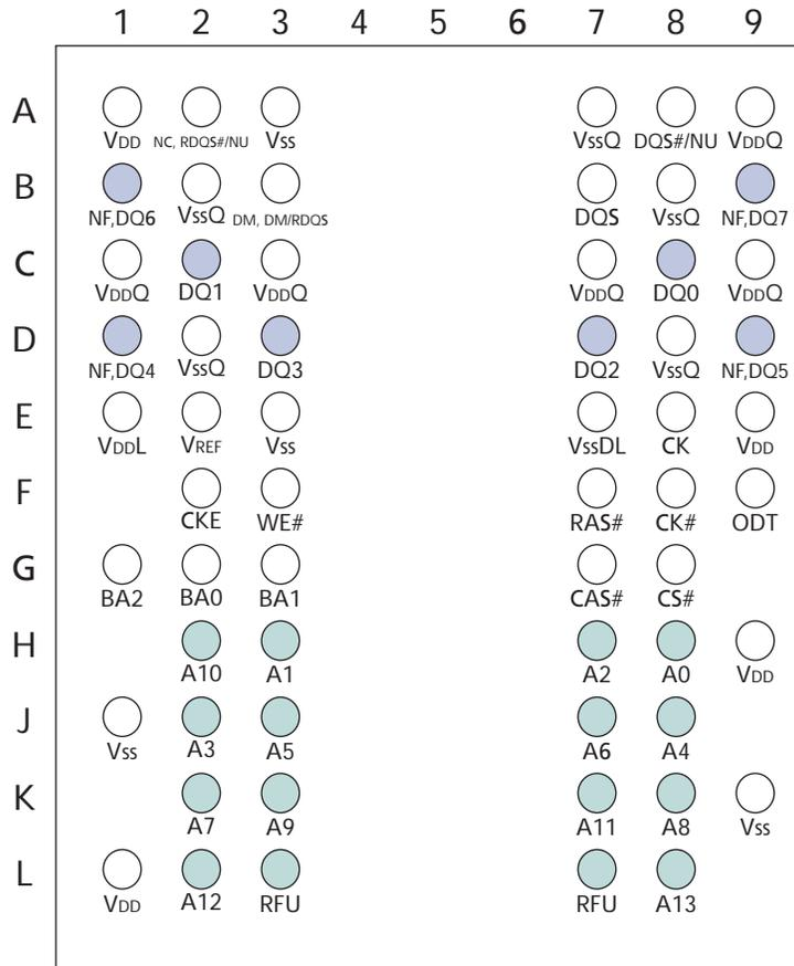
**Figure 7: 84-Ball FBGA – x16 Ball Assignments (Top View)**
