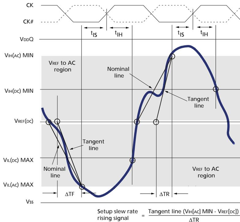
Figure 27: Nominal Slew Rate for  $t_{IH}$
