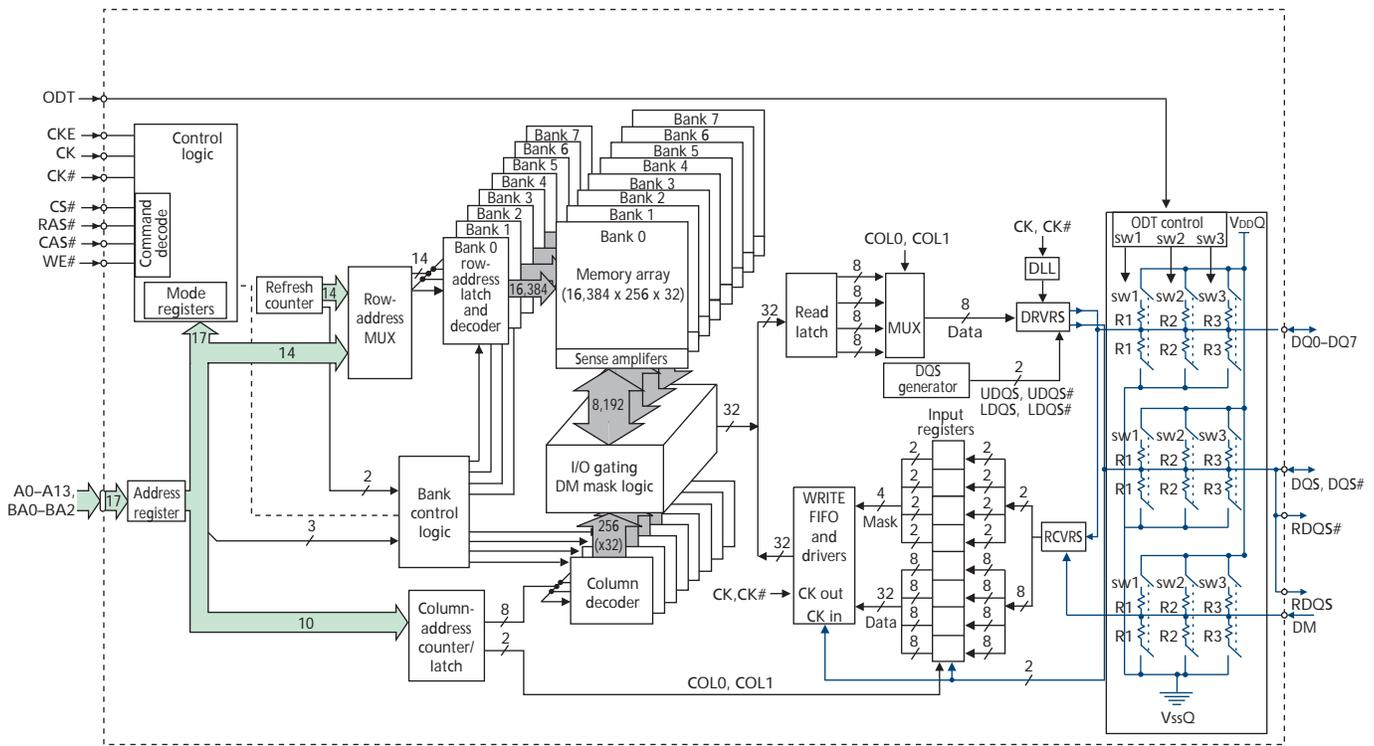
Figure 5: 64 Meg x 16 Functional Block Diagram
