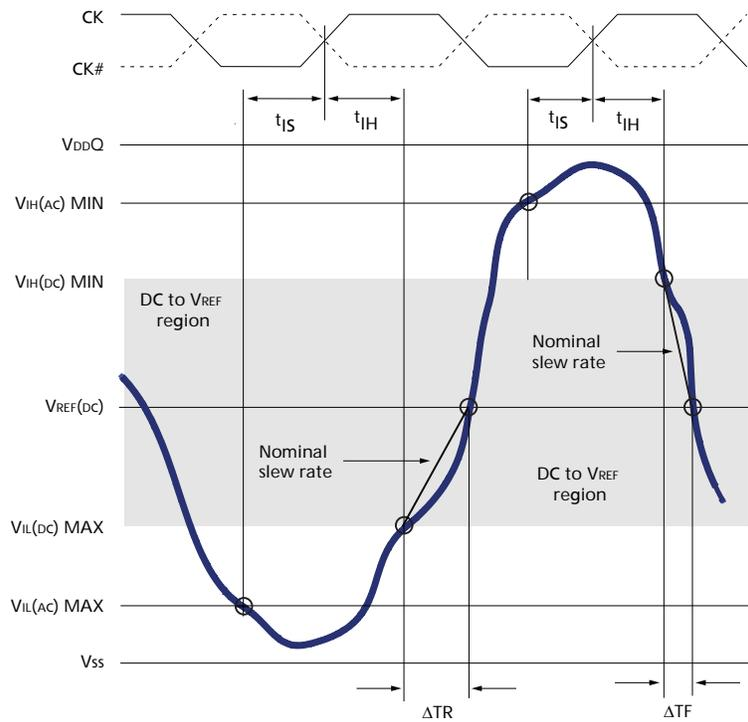
Figure 28: Tangent Line for  $t_{IH}$
