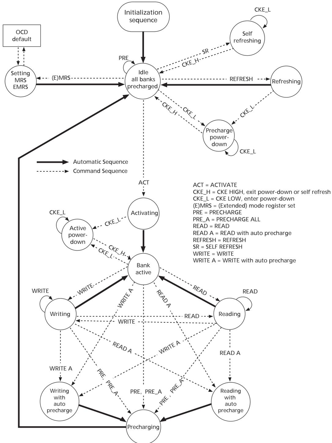
Notes: 1. This diagram provides the basic command flow. It is not comprehensive and does not identify all timing requirements or possible command restrictions such as multibank interaction, power down, entry/exit, etc.
