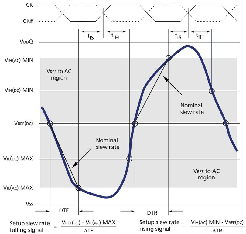
Figure 26: Tangent Line for  $t_{IS}$
