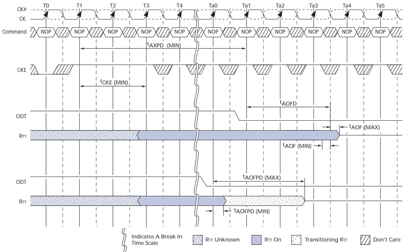
Figure 90: ODT Turn-On Timing When Exiting Power-Down Mode
