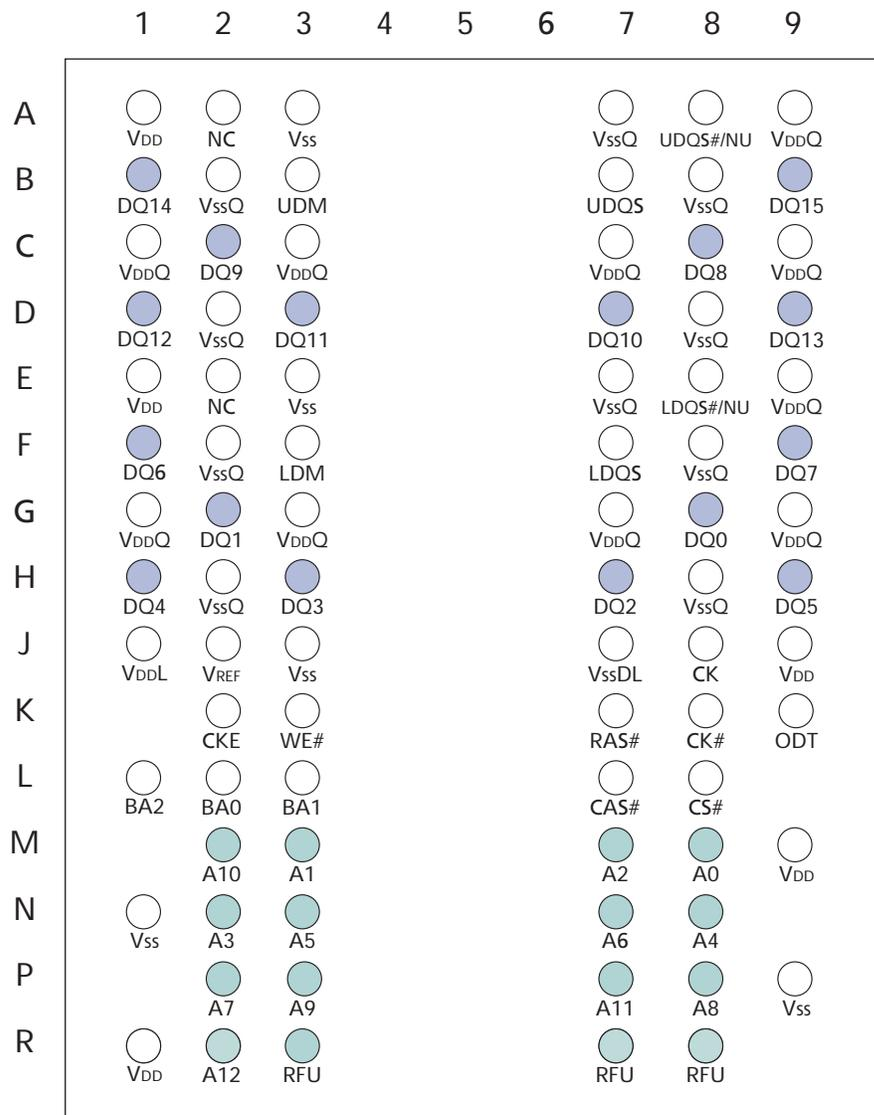
Figure 8: 92-Ball FBGA – x4, x8 Ball Assignments (Top View)
