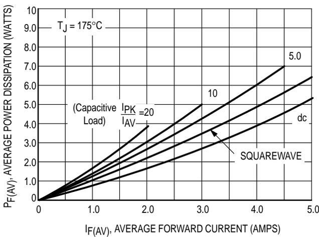
Figure 4. Power Dissipation
