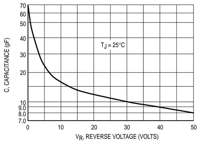
Figure 5. Typical Capacitance
