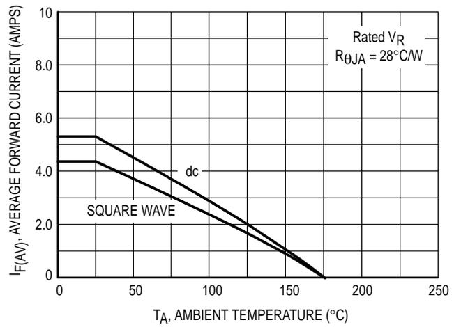
Figure 3. Current Derating (Mounting Method #3 Per Note 1)
