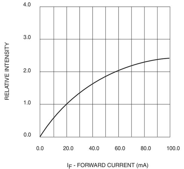
**Fig. 2 Relative Luminous Intensity vs. Forward Current**
