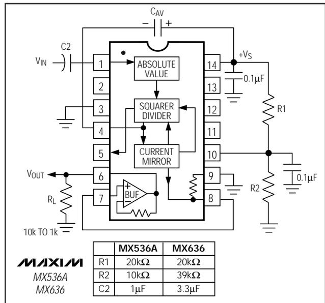
Figure 5. Single-Supply Operation
