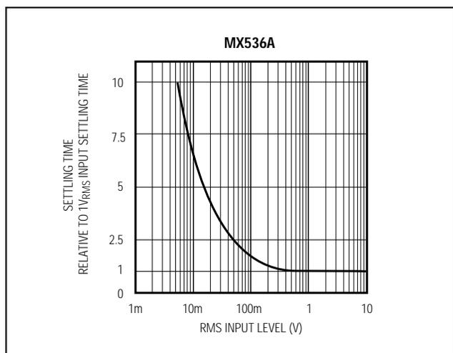
Figure 6a. MX536A Settling Time vs. Input Level
