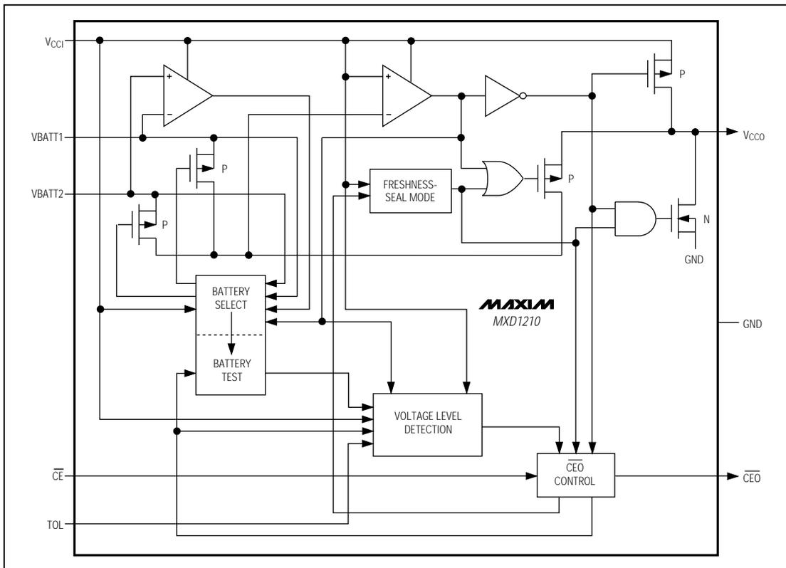
Figure 1. Block Diagram
