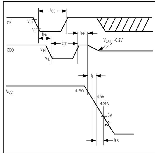
Figure 3. Power-Down Timing Diagram
