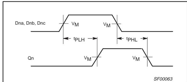
Waveform 2. Propagation Delay for Non-Inverting Outputs (74F11)
