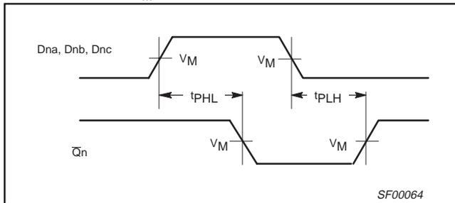
Waveform 1. Propagation Delay for Inverting Outputs (74F10)
