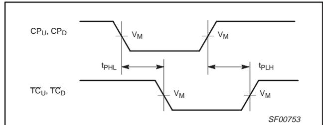
**Waveform 2. Propagation Delay, Clock to Terminal Count**
