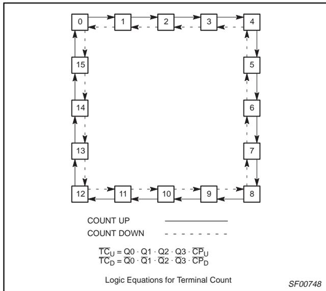
Up/down binary counter with separate up/down clocks
