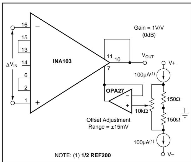
FIGURE 4. Output Offsetting.
