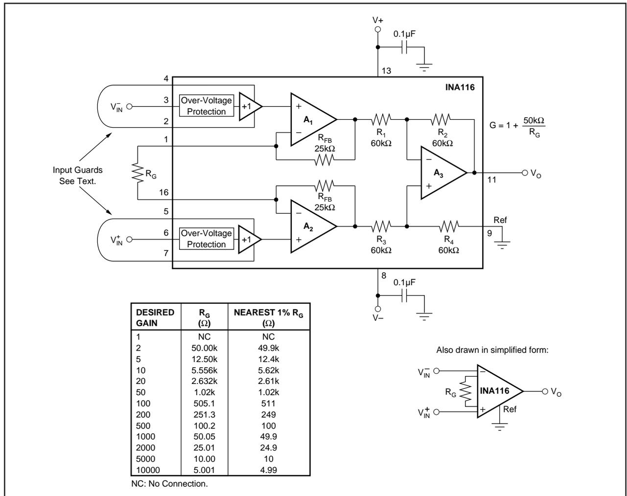
FIGURE 1. Basic Connections.
