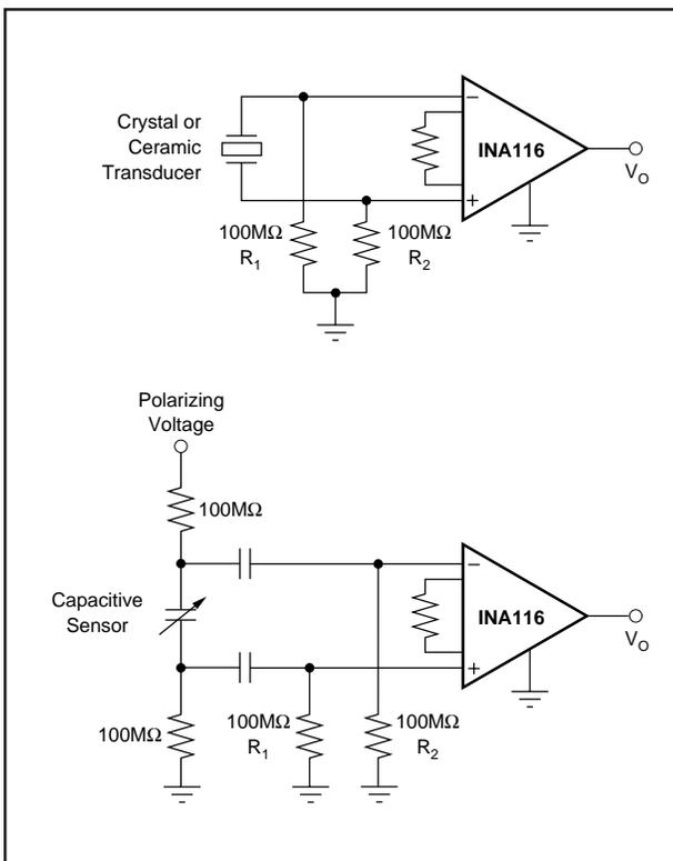
FIGURE 3. Providing An Input Bias Current Path.
