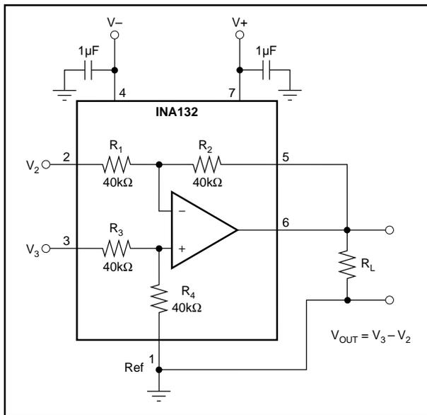
FIGURE 1. Basic Power Supply and Signal Connections.
