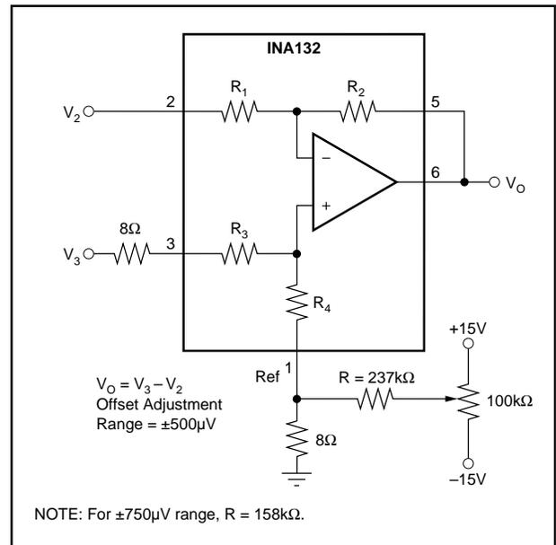
FIGURE 2. Offset Adjustment.
