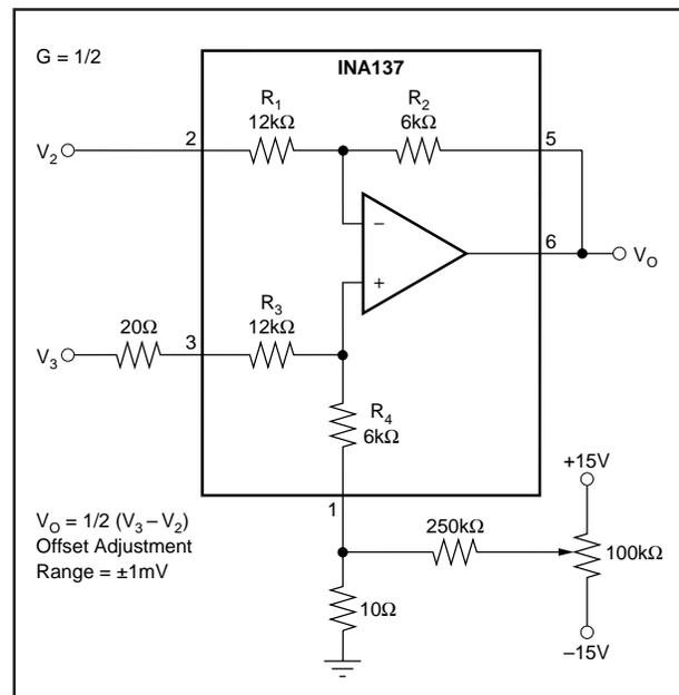
FIGURE 3. Offset Adjustment.
