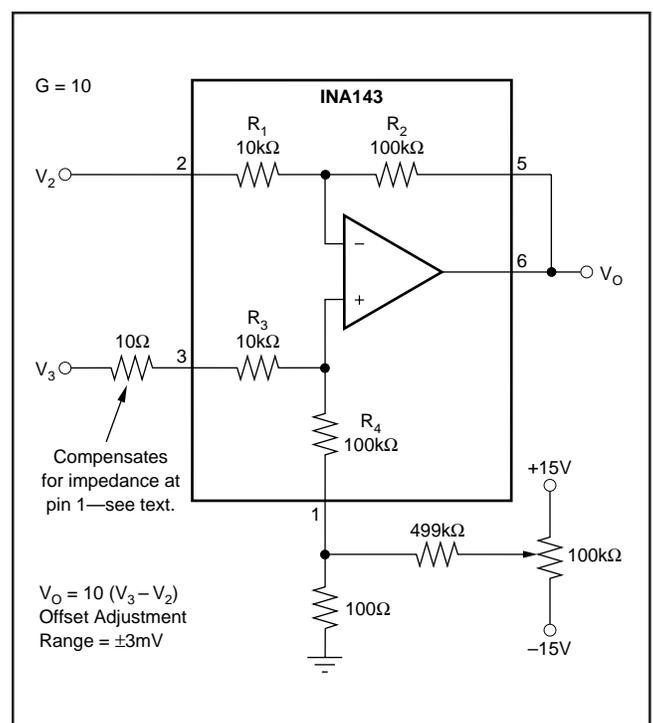
FIGURE 3. Offset Adjustment.
