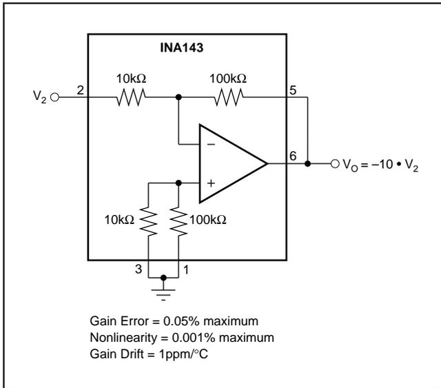
FIGURE 5. Precision  $G = -10$  Inverting Amplifier.
