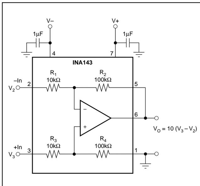
FIGURE 1.  $G = 10$  Basic Power Supply and Signal Connections.
