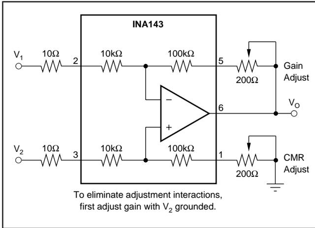
FIGURE 4. Difference Amplifier with Gain and CMR Adjust.
