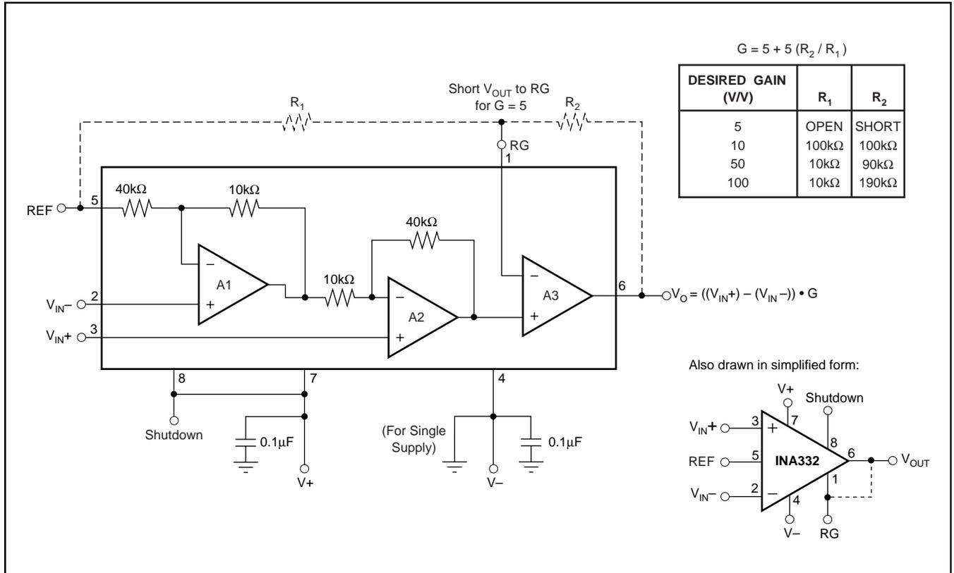
FIGURE 1. Basic Connections.
