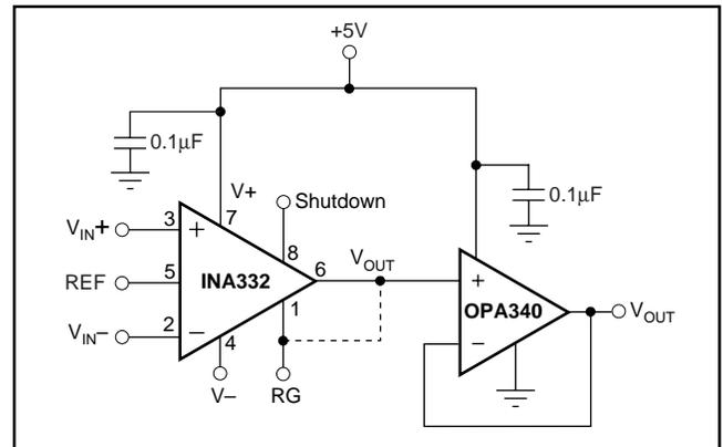
FIGURE 5. Output Buffering Circuit. Able to drive loads as low as 600Ω.
