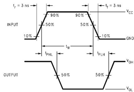
FIGURE 12. AC Waveforms
