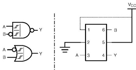
FIGURE 3. 2-Input NAND with Inverted B Input
