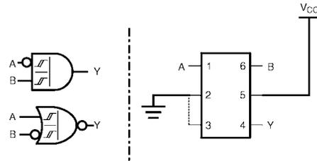
FIGURE 7. 2-Input AND with Inverted A Input
