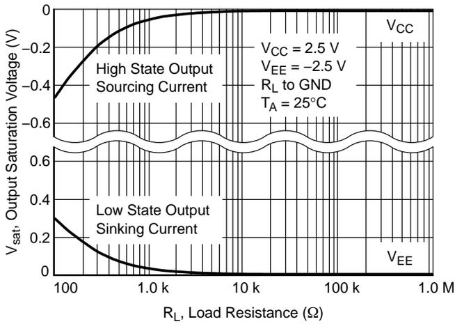
**Figure 2. Split Supply Output Saturation vs. Load Resistance**
