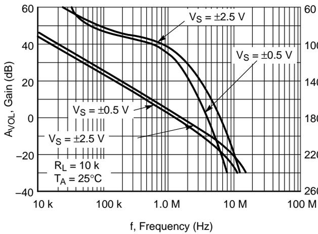
Figure 20. Voltage Gain and Phase vs. Frequency
