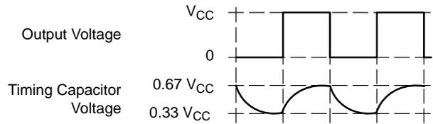
The non-inverting input threshold levels are set so that the capacitor voltage oscillates between 1/3 and 2/3 of  $V_{CC}$ . This requires the resistors  $R_{1a}$ ,  $R_{1b}$  and  $R_2$  to be of equal value. The following formula can be used to approximate the output frequency.
