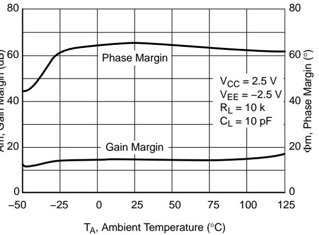
Figure 21. Gain and Phase Margin vs. Temperature
