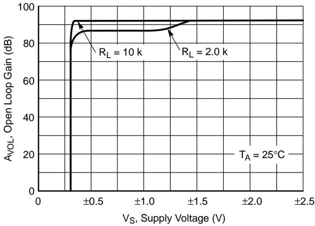
**Figure 26. Open Loop Voltage Gain vs. Supply Voltage**
