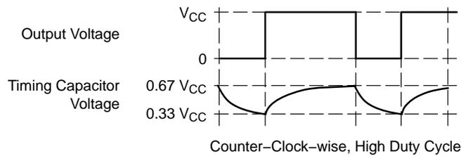
The timing capacitor  $C_T$  will charge through diode  $D_2$  and discharge through diode  $D_1$ , allowing a variable duty cycle. The pulse width of the signal can be programmed by adjusting the value of the trimpot. The capacitor voltage will oscillate between 1/3 and 2/3 of  $V_{CC}$ , since all the resistors at the non-inverting input are of equal value.
