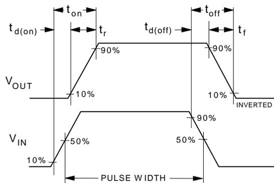
Figure 12. Switching Waveforms.
