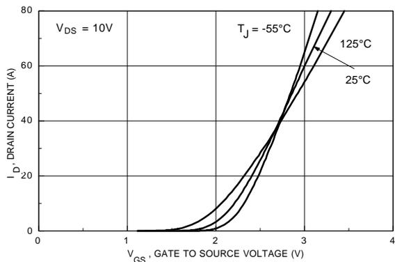
Figure 5. Transfer Characteristics.
