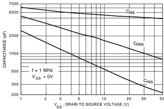
Figure 9. Capacitance Characteristics.
