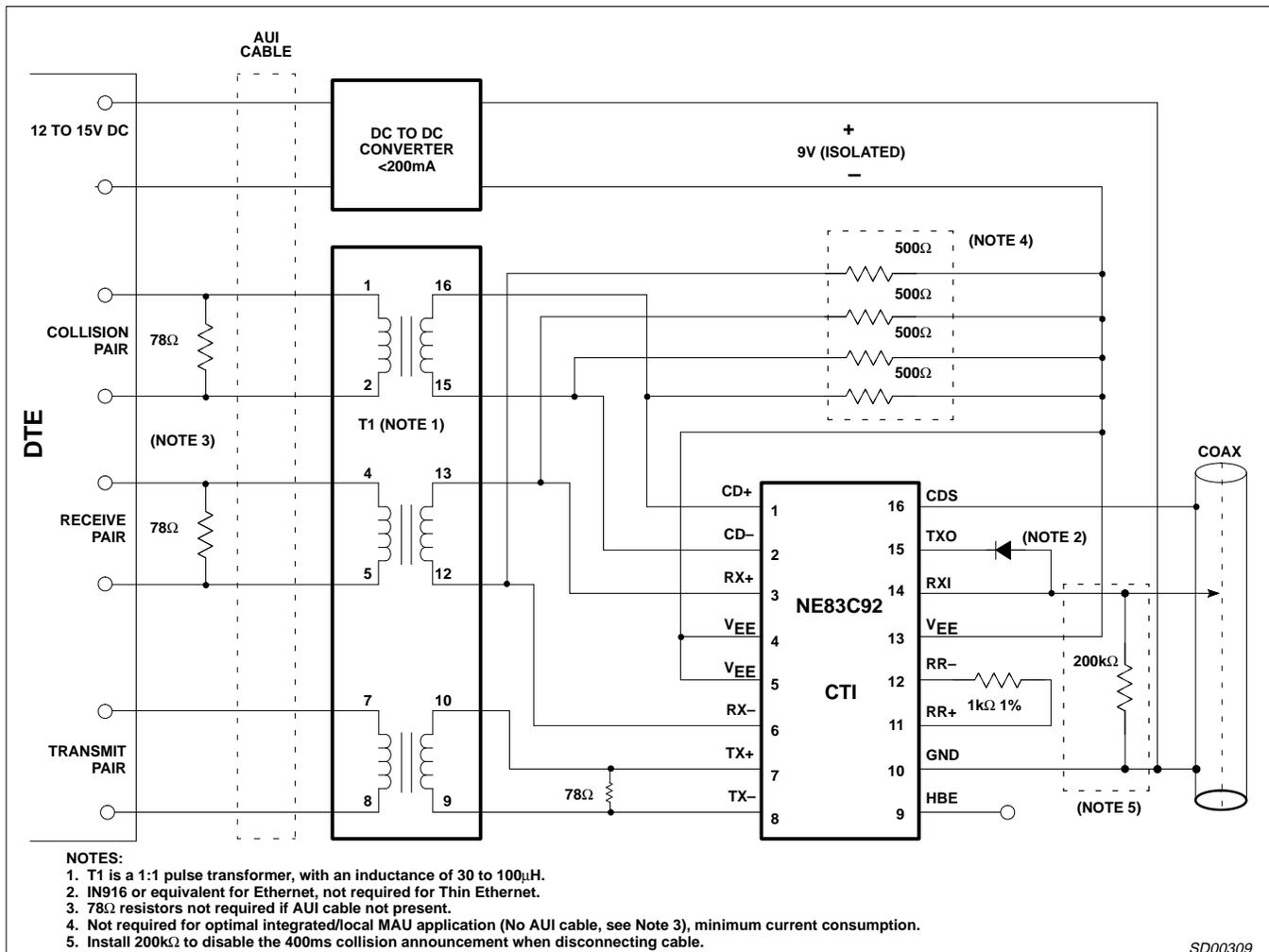
Figure 1. Connection Diagram for Standard 8392 Applications
