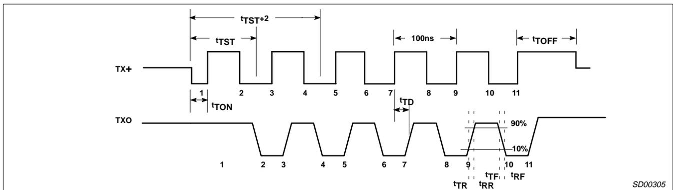
Figure 5. Transmitter Timing
