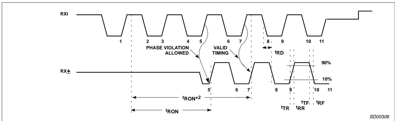
Figure 3. Receiver Timing
