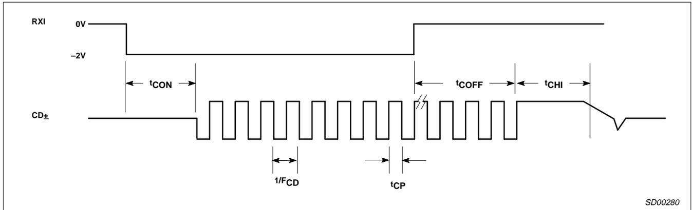
Figure 6. Collision Timing
