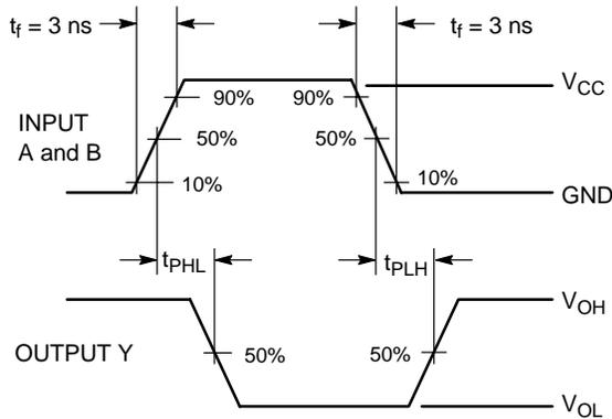
Figure 3. Switching Waveforms
