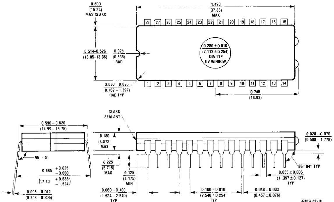
**UV Window Cavity Dual-In-Line Package (J)
