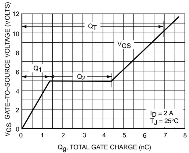
Figure 8. Gate-to-Source and Drain-to-Source Voltage versus Total Charge
