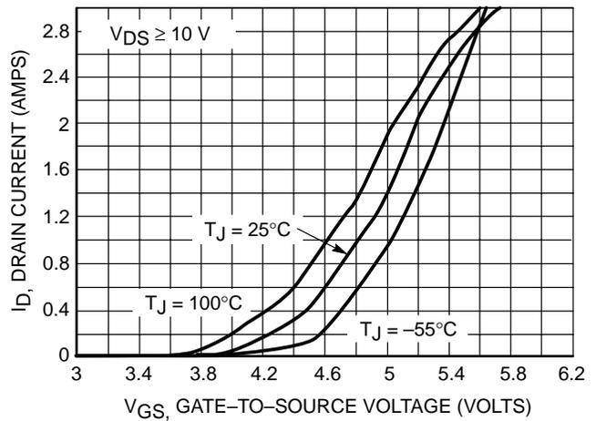
Figure 2. Transfer Characteristics
