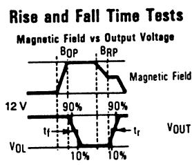
Rise and Fall Time Test Circuit
