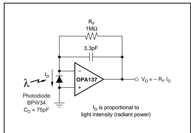
FIGURE 3. Photodetector Amplifier.
