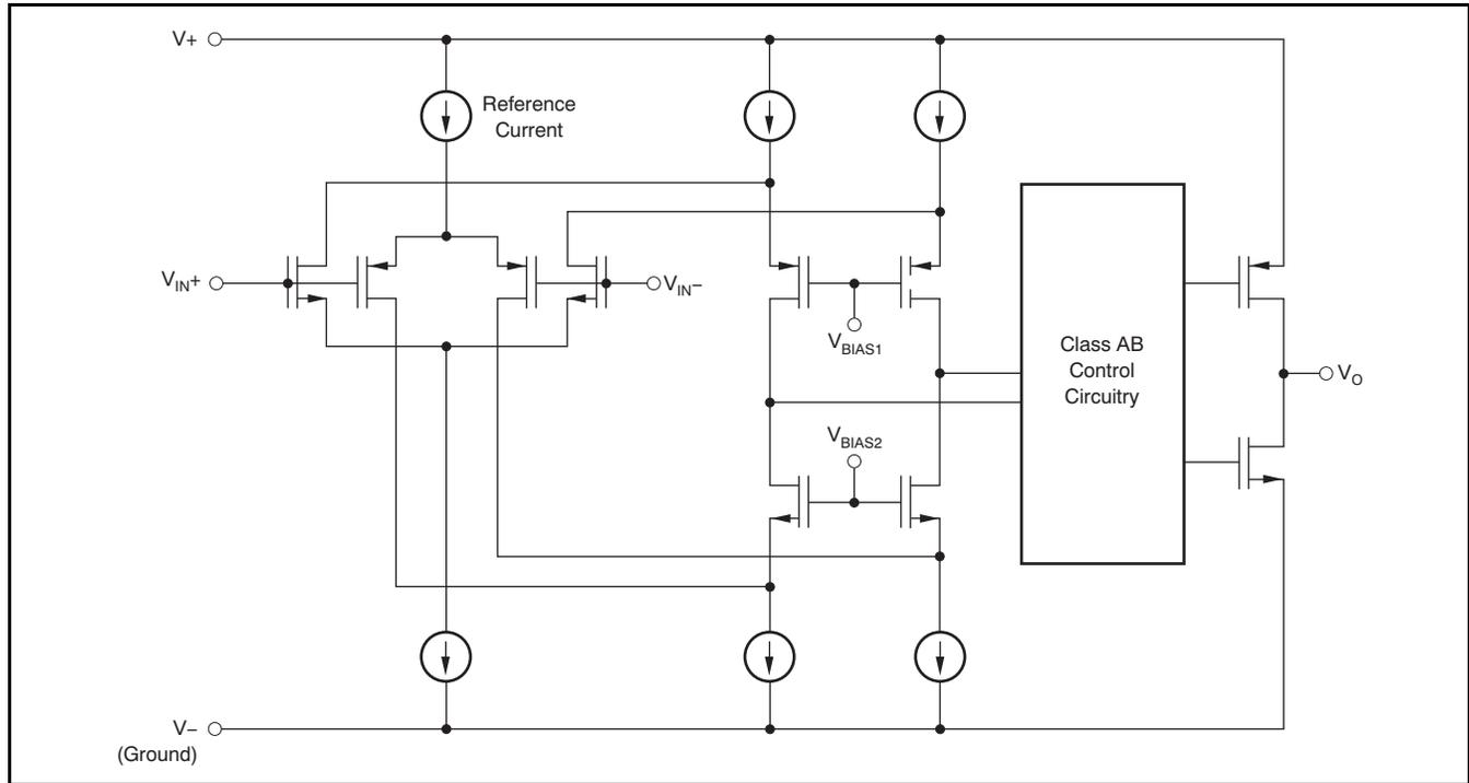
Figure 24. Simplified Schematic
