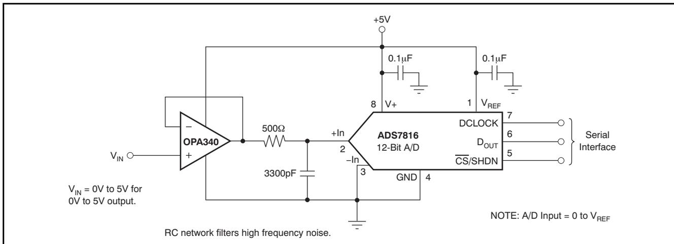
Figure 27. OPA340 in Noninverting Configuration Driving ADS7816
