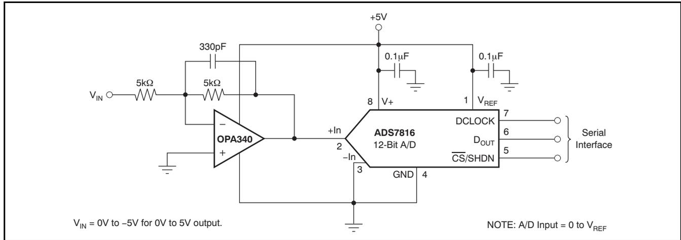
Figure 28. OPA340 in Inverting Configuration Driving ADS7816
