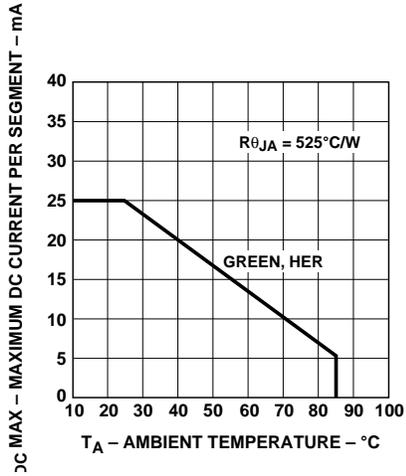
Figure 1. Maximum Allowable DC Current vs. Ambient Temperature.
